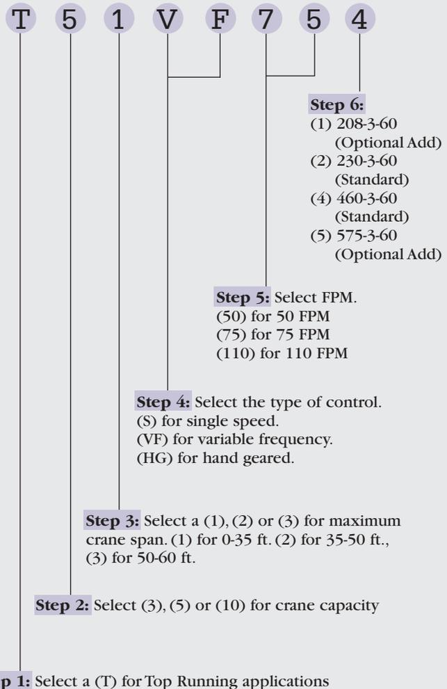
Our example shows a Top Running crane with a 5 ton capacity and a 0-35 foot span. It has variable frequency controls, can travel 75 feet per minute, and is set for 460 volt.
