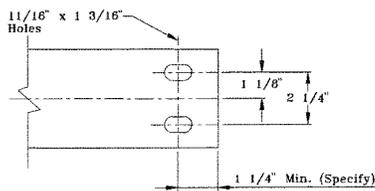
The D-60 pattern is used at all support points of light rail tracks for bolted or flush clamped track suspensions.
