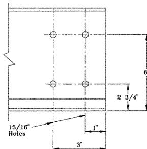
The W-30 preparation is for the No. 340130 track coupling. It is used for coupling Nos. 34011 and 34016 track.
