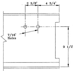
The W-75 pattern is for the No. 550315 conductor bar support. It is used when Type H interlocks are electrified and bottom of conductor is 7-3/4" above tread.
