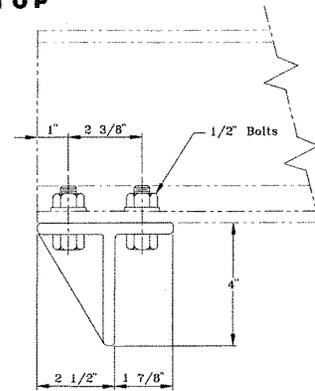
Use for hand propelled or motor driven carriers and cranes with 6-1/2" diameter wheels.
