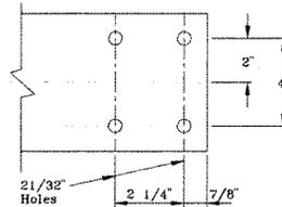
The D-50 pattern is for the No. 4504 guide roller and is used at track ends having an interlock.
