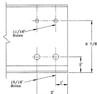
The W-32 preparation is for the No. 340132 track coupling. It is used for coupling Nos. 34037, 34041 and 34046 track.
