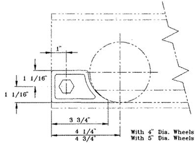
Use for hand propelled carriers and cranes with 4" or 5" diameter wheels.
