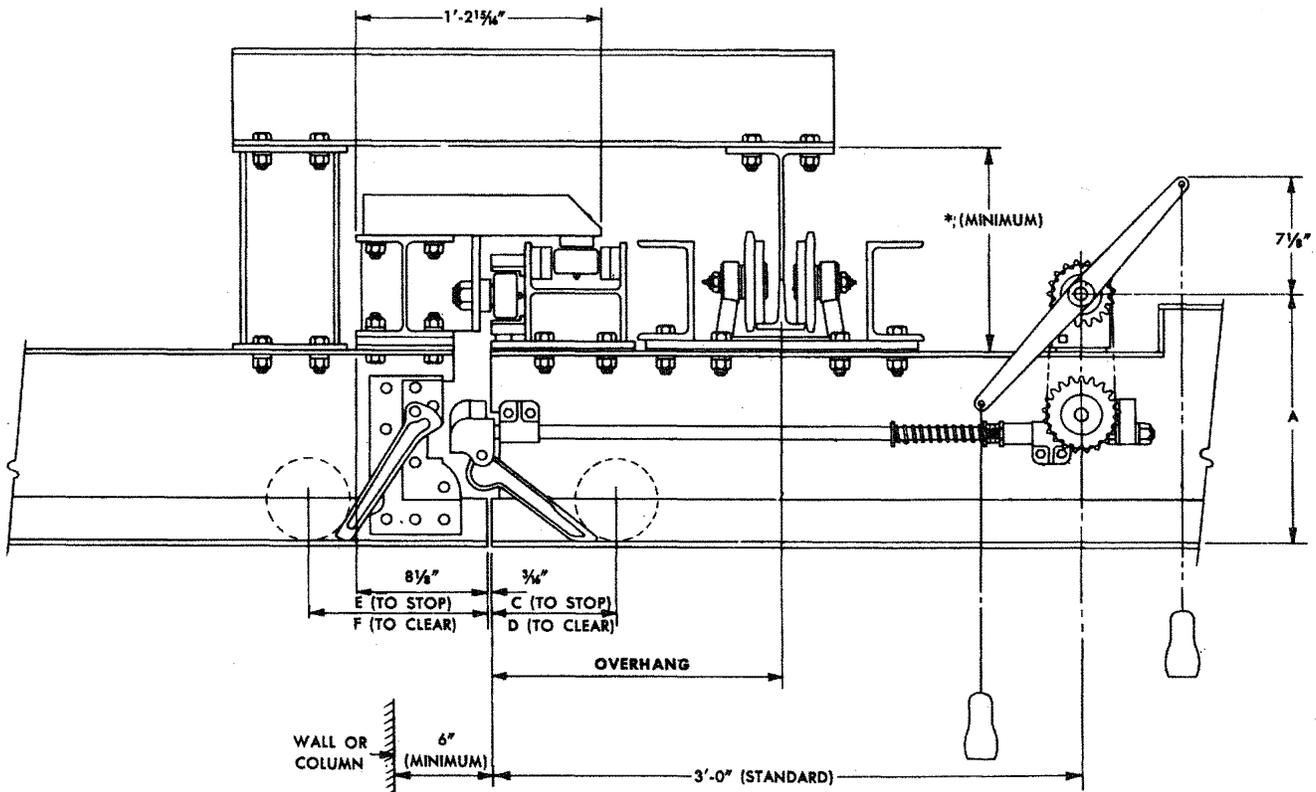
\*11-1/2 inch minimum with 5 inch wheel end trucks; 14 inch minimum with 6-1/2 inch or 8 inch wheel end trucks.
