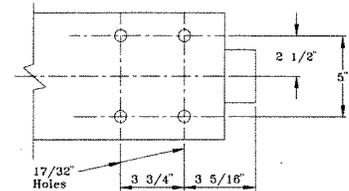
The D-68 pattern is for the No. 4501005 lower guide and is used at track ends having a discharge point.
