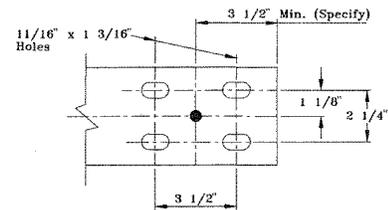
The D-108 pattern is for the No. 340110 track hanger. It is used at end or intermediate support points for single 3/4" rod suspension of No. 34011 (8") track.
