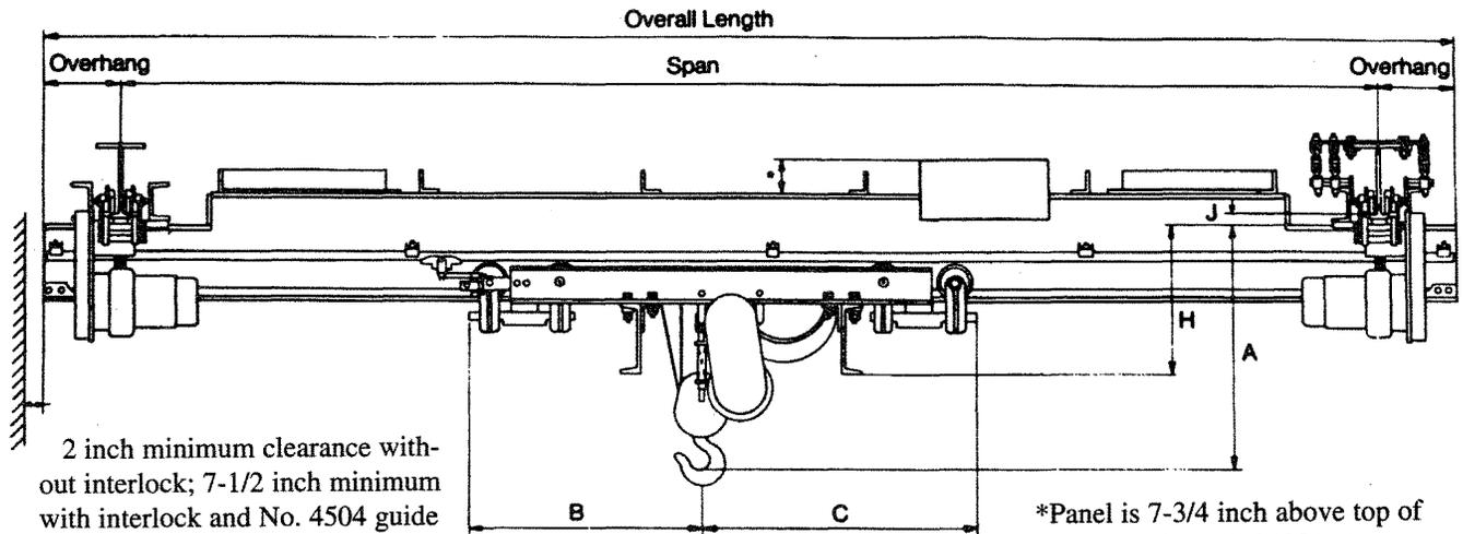
2 inch minimum clearance without interlock; 7-1/2 inch minimum with interlock and No. 4504 guide roller; or 6 inch minimum with interlock and No. 45090 guide.
