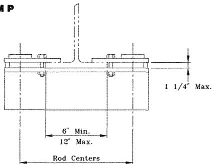
**NO. 340105 BEAM CLAMP - 17,000 LBS. RATED LOAD
