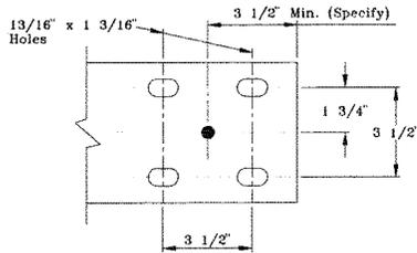
The D-105 pattern is for the No. 340123 track hanger and No. 340125 top splice plate. It is used at end or intermediate support points for single 1-1/8" rod suspensions and at all support points for double 1-1/8" rod suspensions with rod centers greater than 7" and less than 12".
