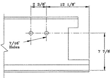
The W-72 pattern is for the No. 550311 conductor bar support. It is used when Type L discharge points are electrified and bottom of conductor is 6-1/8" above tread.
