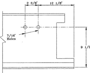
The W-73 pattern is for the No. 550311 conductor bar support. It is used when Type H discharge points are electrified and bottom of conductor is 7-3/4" above tread.
