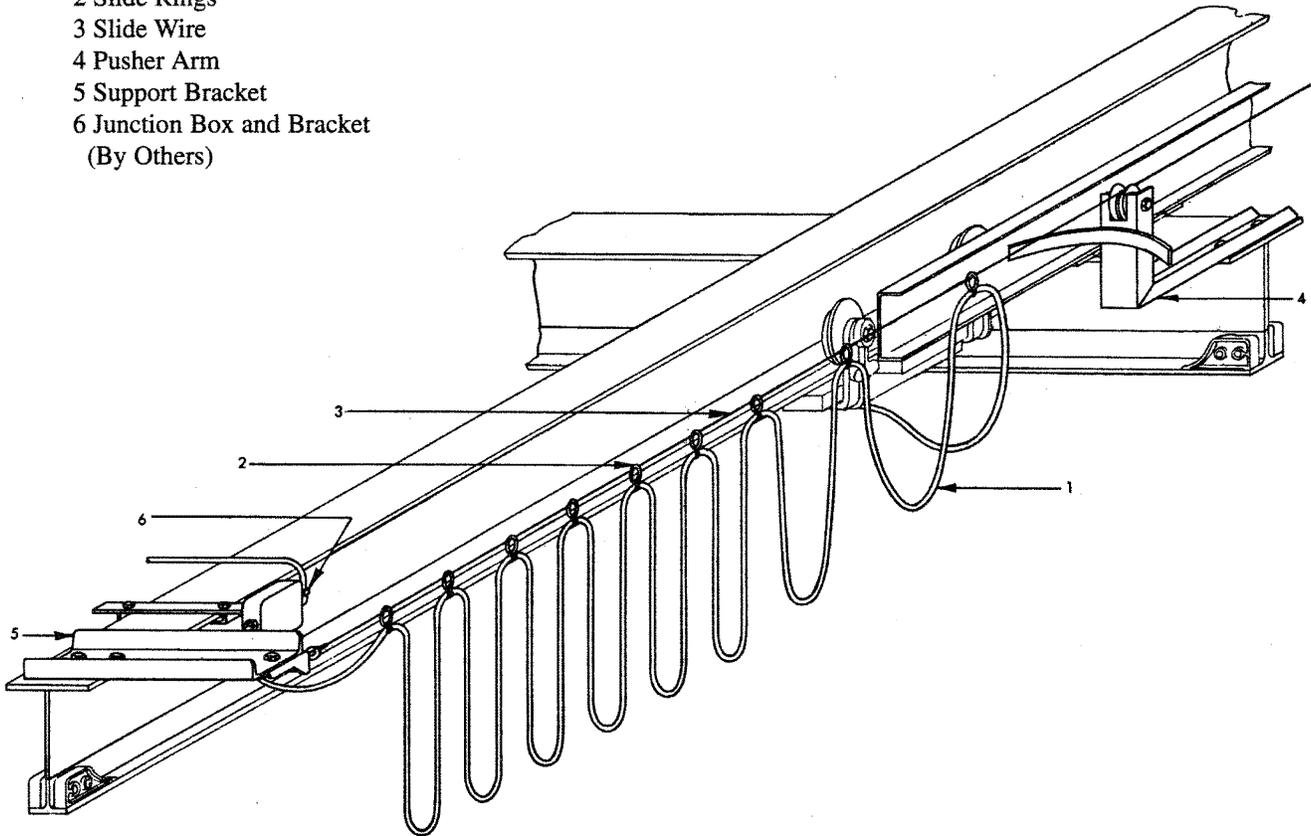
Tagline electrification uses flexible cable for the conductors. It is well suited for applications in hazardous locations or where there are corrosive fumes or high humidity in the atmosphere. Tagline is not generally used on systems with curves, switches or interlocks.
