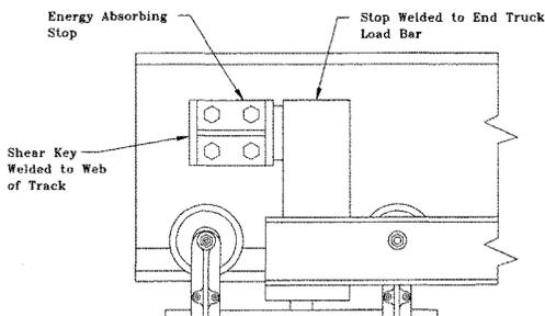
The stop illustrated is one of several available. Energy is absorbed by a rubber pad bonded to the stop. Polyurethane and spring stops are also available. Consult factory for recommendations on applications requiring energy absorbing stops.
