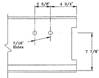
The W-74 pattern is for the No. 550315 conductor bar support. It is used when Type L interlocks are electrified and bottom of conductor is 6-1/8" above tread.
