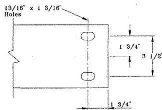
The D-107 pattern is for the No. 340126 top splice plate. It is used at coupling support points for double 1-1/8" rod suspensions with rod centers of 12" or more.
