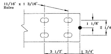
The D-104 pattern is for the No. 340110 track hanger and No. 340112 top splice plate. It is used at coupling support points for single 3/4" rod suspensions of No. 34011 (8") track.
