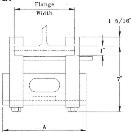
**NO. 340102 BEAM CLAMP - 8,500 LBS. RATED LOAD**
