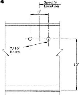
The W-114 pattern is for the No. 550496 conductor bar support. It is used on Nos. 34061 through 34079 track when carriers or cranes have 5", 6-1/2" or 8" diameter wheels and bottom of conductor is 11-7/8" above tread.
