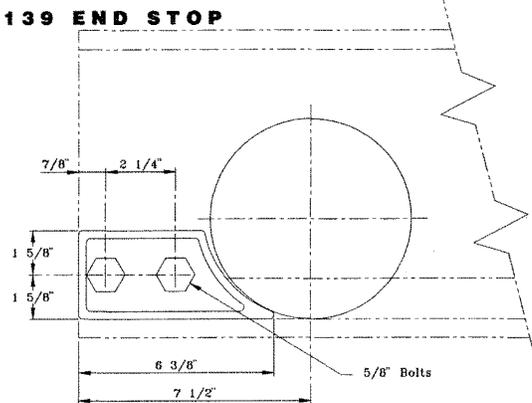
Use for hand propelled or motor driven carriers and cranes with 6-1/2" diameter wheels.
