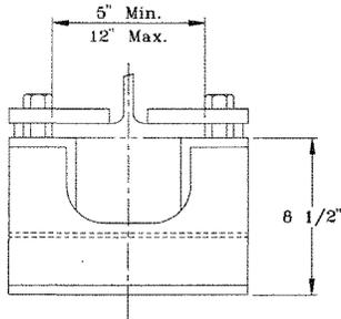
**NO. 340117 BEAM CLAMP - 20,000 LBS. RATED LOAD**
