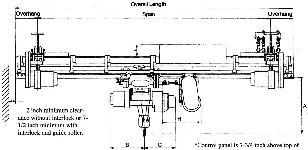
\*Control panel is 7-3/4 inch above top of Nos. 34021 through 34056 girders. Panel is below top of girder for No. 34061 and larger girders.
