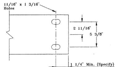
The D-61 pattern is used at all support points of heavy rail tracks for bolted or flush clamped track suspensions.
