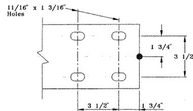
D-102 pattern is for the No. 340111 track hanger and No. 340113 top splice plate. It is used at coupling support points for single 3/4" rod suspensions and double 3/4" rod suspensions with 7" rod centers.
