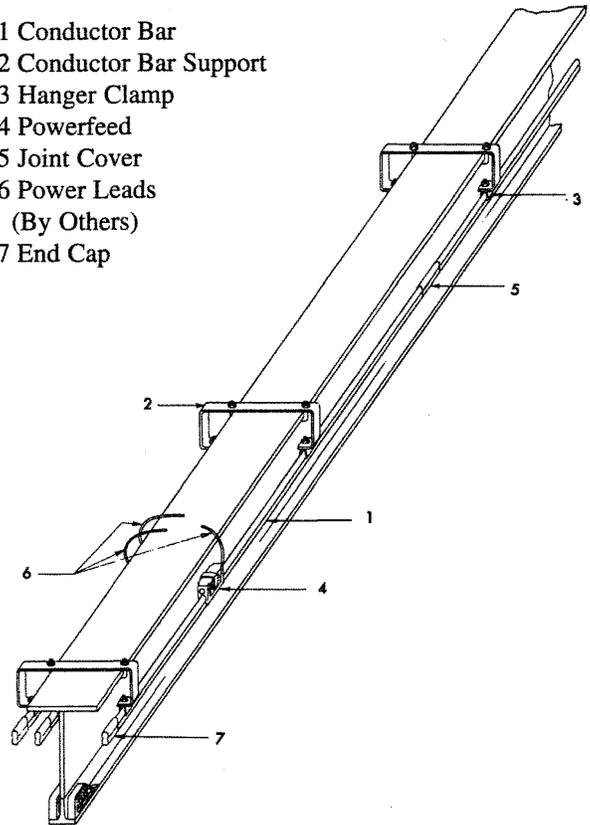
Powerfeeds provide taps for connecting the power and control sources to the conductor. They clamp to the upper lobe of the conductor and can be installed at any point along the conductor.
