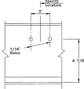
The W-56 pattern is for the No. 550341 conductor bar support. It is used on Nos. 34051 through 34079 track when carriers or cranes have 6-1/2" diameter wheels and bottom of conductor is 7-3/4" above tread.
