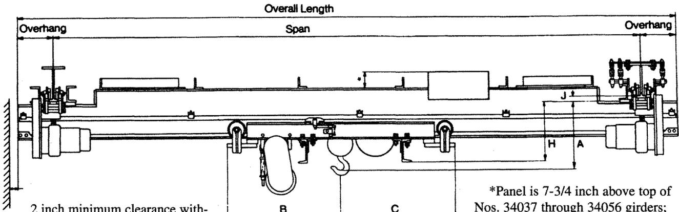
2 inch minimum clearance without interlock; 7-1/2 inch minimum with interlock and No. 4504 guide roller; or 6 inch minimum with interlock and No. 45090 guide.
