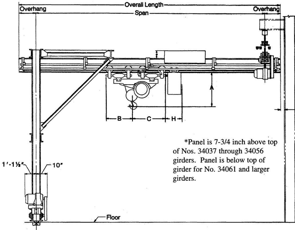
2 inch minimum clearance without interlock or 7-1/2 inch minimum with interlock and guide roller.
