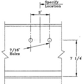
The W-55 pattern is for the No. 550341 conductor bar support. It is used on Nos. 34051 through 34079 track when carriers or cranes have 4" or 5" diameter wheels and bottom of conductor is 6-1/8" above tread.
