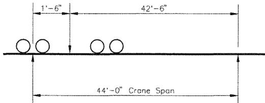
**STEP 4 - Determine end truck wheelbase dimensions from Crane Section.**
