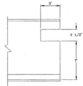
The W-91 preparation is used on the ends of all straight and curve tracks incoming to Types 4 and 5 electrified switches when bottom of conductor is 7-3/4" above tread.
