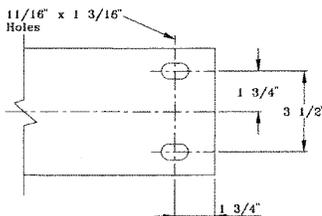
The D-103 pattern is for the No. 340115 top splice plate. It is used at coupling support points for double 3/4" rod suspensions with rod centers of 12" or more.
