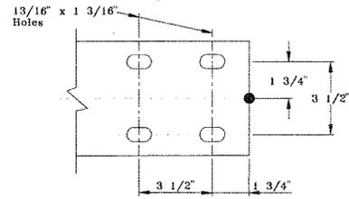
The D-106 pattern is for the No. 340123 track hanger and No. 340124 top splice plate. It is used at coupling support points for single 1-1/8" rod suspensions and double 1-1/8" rod suspensions with 7" rod centers.
