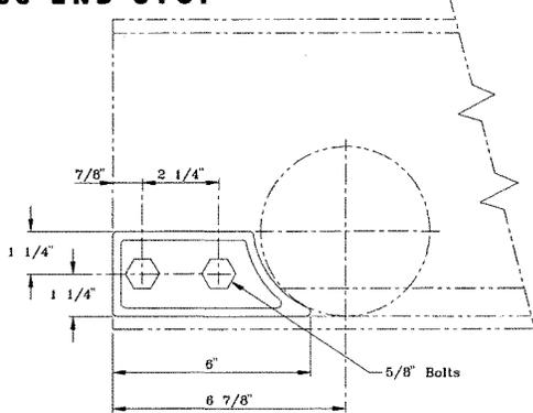
Use for hand propelled or motor driven carriers and cranes with 5" diameter wheels.
