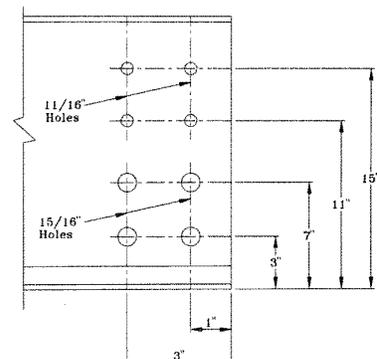
The W-33 preparation is for the No. 340133 track coupling. It is used for coupling Nos. 34051, 34056, 34061 and 34066 track.
