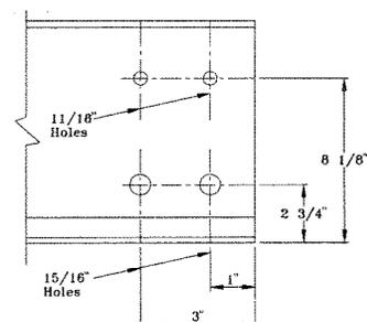
The W-31 preparation is for the No. 340131 track coupling. It is used for coupling Nos. 34021, 34026 and 34031 track.
