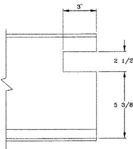
The W-90 preparation is used on the ends of all straight and curve tracks incoming to Types 4 and 5 electrified switches when bottom of conductor is 6-1/8" above tread.
