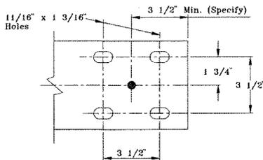
The D-101 pattern is for the No. 340111 track hanger and No. 340114 top splice plate. It is used at end or intermediate support points for single 3/4" rod suspensions and at all support points for double 3/4" rod suspensions with rod centers greater than 7" and less than 12".
