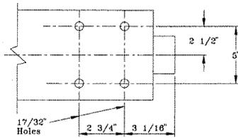
The D-38 pattern is for the No. 4501007 guide roller guide and is used at track ends having a discharge point.
