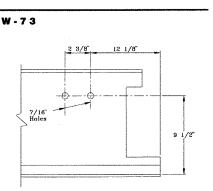
The W-73 pattern is for the No. 550311 conductor bar support. It is used when Type H discharge points are electrified and bottom of conductor is 7-3/4" above tread.
