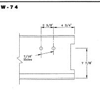
The W-74 pattern is for the No. 550315 conductor bar support. It is used when Type L interlocks are electrified and bottom of conductor is 6-1/8" above tread.
