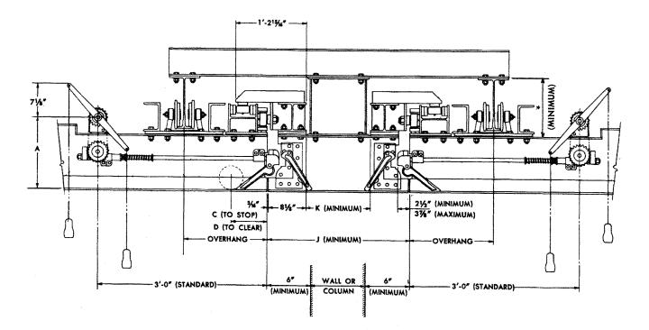
\*11-1/2 inch minimum with 5 inch wheel end trucks; 14 inch minimum with 6-1/2 inch or 8 inch wheel end trucks.
