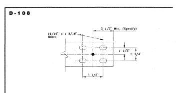
The D-108 pattern is for the No. 340110 track hanger. It is used at end or intermediate support points for single 3/4" rod suspension of No. 34011 (8") track.
