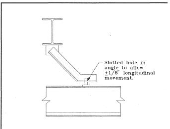
Longitudinal bracing using a steel pin engaging a slotted hole in a steel angle.
