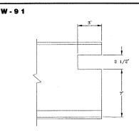
The W-91 preparation is used on the ends of all straight and curve tracks incoming to Types 4 and 5 electrified switches when bottom of conductor is 7-3/4" above tread.
