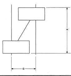
Close grouping of switches may require outriggers for remote operation of the control ropes to avoid interference between the ropes on one switch and a carrier leaving an adjacent switch. Consult factory for information on outriggers and remote operation.
