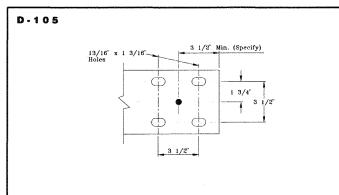
The D-105 pattern is for the No. 340123 track hanger and No. 340125 top splice plate. It is used at end or intermediate support points for single 1-1/8" rod suspensions and at all support points for double 1-1/8" rod suspensions with rod centers greater than 7" and less than 12".
