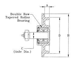
Double Row Tapered Roller Bearing C (Axle Dia.)
