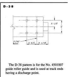
TOP FLANGE DRILLING AND PUNCHING PATTERNS
