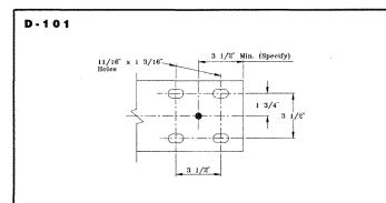
The D-101 pattern is for the No. 340111 track hanger and No. 340114 top splice plate. It is used at end or intermediate support points for single 3/4" rod suspensions and at all support points for double 3/4" rod suspensions with rod centers greater than 7" and less than 12".
