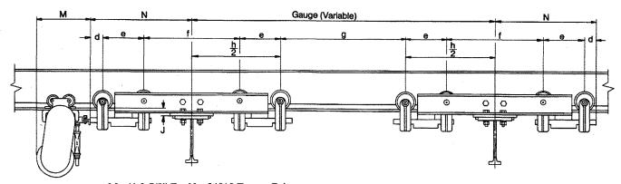
M= 1'-3-7/8" For No. 24010 Tractor Drive 1'-2-1/2" For No. 2409 Tractor Drive 1'-11-1/4" For No. 2408 Tractor Drive
