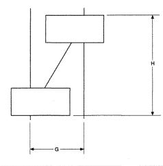
Close grouping of switches may require outriggers for remote operation of the control ropes to avoid interference between the ropes on one switch and a carrier leaving an adjacent switch. Consult factory for information on outriggers and remote operation.
