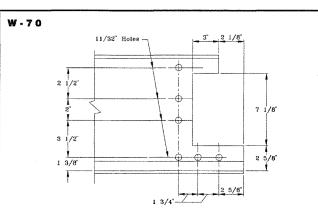
The W-70 preparation is for the Type L discharge point. It is used on all track sizes. Nos. 34011, 34016 and 34021 must be built up to 11-1/2" depth to accommodate this preparation.
