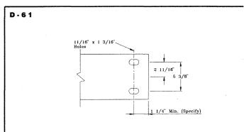
The D-61 pattern is used at all support points of heavy rail tracks for bolted or flush clamped track suspensions.
