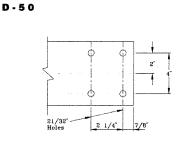
The D-50 pattern is for the No. 4504 guide roller and is used at track ends having an interlock.
