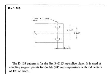
applied to curves. Patterns for track hangers are dimensioned to the center of the hanger rod and from one end using an end with a coupling preparation as the starting point.
