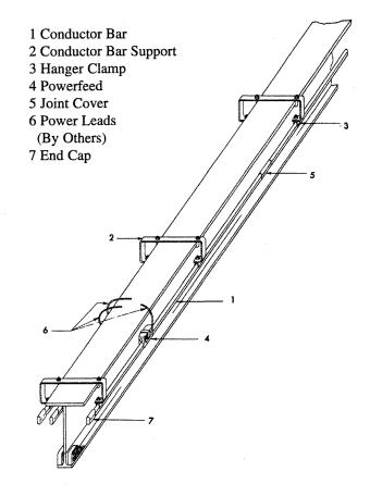
Powerfeeds provide taps for connecting the power and control sources to the conductor. They clamp to the upper lobe of the conductor and can be installed at any point along the conductor.
