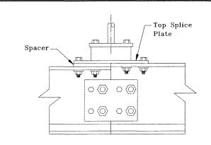
Coupling arrangement with single hanger rod suspension and smaller track spaced to the depth of the larger track. This arrangement is generally used where the difference in track depths is 1-1/2" or less.
