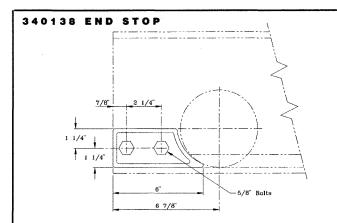
Use for hand propelled or motor driven carriers and cranes with 5" diameter wheels.
