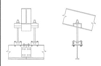
Double rod suspension using a special beam saddle welded to the lower flange and web of the rigid frame.
