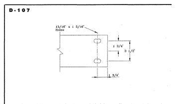
The D-107 pattern is for the No. 340126 top splice plate. It is used at coupling support points for double 1-1/8" rod suspensions with rod centers of 12" or more.
