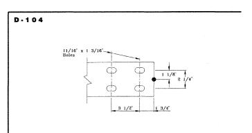
The D-104 pattern is for the No. 340110 track hanger and No. 340112 top splice plate. It is used at coupling support points for single 3/4" rod suspensions of No. 34011 (8") track.
