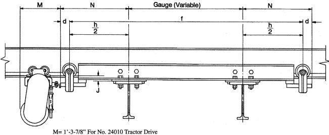
M= 1'-3-7/8" For No. 24010 Tractor Drive 1'-2-1/2" For No. 2409 Tractor Drive 1'-11-1/4" For No. 2408 Tractor Drive
