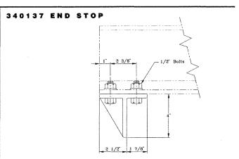
Use for hand propelled or motor driven carriers and cranes with 6-1/2" diameter wheels.
