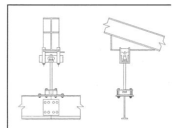
Single rod suspension using a beam clamp clamped to a horizontal bracket supplied with the rigid frame.
