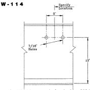
The W-114 pattern is for the No. 550496 conductor bar support. It is used on Nos. 34061 through 34079 track when carriers or cranes have 5", 6-1/2" or 8" diameter wheels and bottom of conductor is 11-7/8" above tread.
