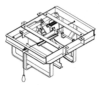
Suspension hardware is not included with the switch and is ordered separately.
