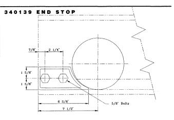
Use for hand propelled or motor driven carriers and cranes with 6-1/2" diameter wheels.
