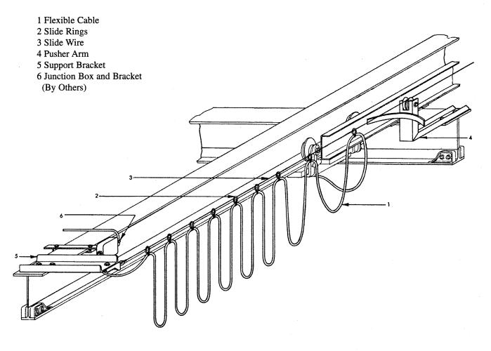
Tagline electrification uses flexible cable for the conductors. It is well suited for applications in hazardous locations or where there are corrosive fumes or high humidity in the atmosphere. Tagline is not generally used on systems with curves, switches or interlocks.
