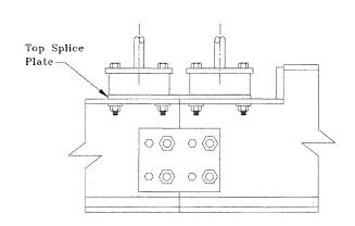
Coupling arrangement with double hanger rod suspension and larger track coped to the depth of the smaller track. This arrangement is generally used where the difference in track depths is 4" or less; consult factory for recommendations when difference is greater than 4".
