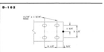
D-102 pattern is for the No. 340111 track hanger and No. 340113 top splice plate. It is used at coupling support points for single 3/4" rod suspensions and double 3/4" rod suspensions with 7" rod centers.
