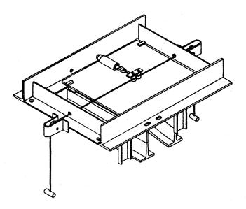
viding adjustment for the incoming tracks. Hardware is included with the switch end preparations for the incoming tracks.
