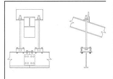
Double rod suspension using a special beam saddle welded to the top flange of the rigid frame.
