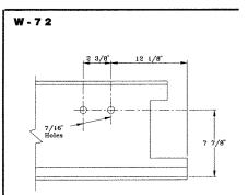
The W-72 pattern is for the No. 550311 conductor bar support. It is used when Type L discharge points are electrified and bottom of conductor is 6-1/8" above tread.
