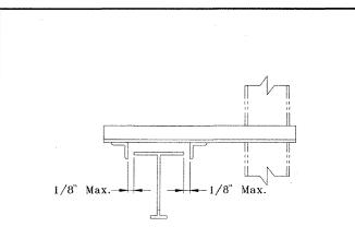
Lateral bracing using steel angles welded to the supporting structure
