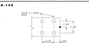
The D-106 pattern is for the No. 340123 track hanger and No. 340124 top splice plate. It is used at coupling support points for single 1-1/8" rod suspensions and double 1-1/8" rod suspensions with 7" rod centers.
