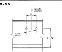
The W-55 pattern is for the No. 550341 conductor bar support. It is used on Nos. 34051 through 34079 track when carriers or cranes have 4" or 5" diameter wheels and bottom of conductor is 6-1/8" above tread.
