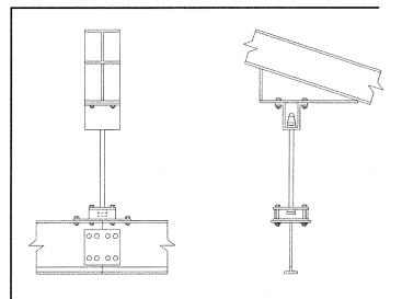
Single rod suspension using a beam cleat bolted to a horizontal bracket supplied with the rigid frame.
