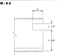
The W-90 preparation is used on the ends of all straight and curve tracks incoming to Types 4 and 5 electrified switches when bottom of conductor is 6-1/8" above tread.
