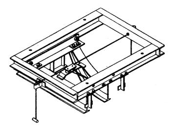
Incoming tracks are bolted to the stationary frame using two 5/8 inch heat treated capscrews, nuts and lockwashers. Slotted holes in the frame help in aligning the system by providing adjustment for the incoming tracks. Hardware is included with the switch end preparations for the incoming tracks.
