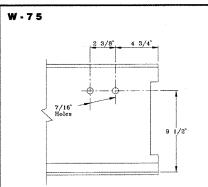
The W-75 pattern is for the No. 550315 conductor bar support. It is used when Type H interlocks are electrified and bottom of conductor is 7-3/4" above tread.
