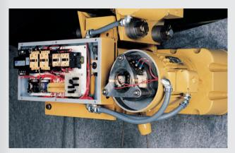
Basic Control Box and Motor Brake
