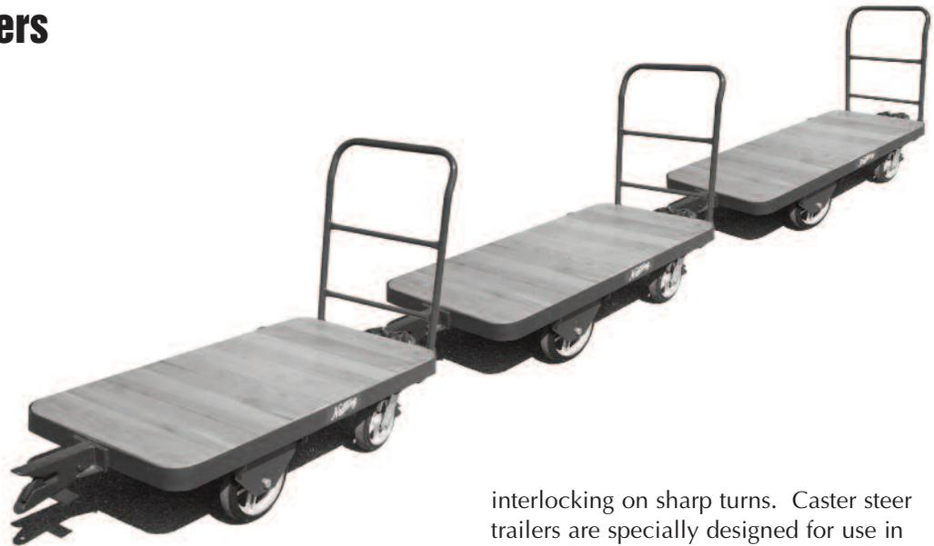
Caster steer trailers turn by swiveling on the front caster wheels. The casters have two full rows of large hardened balls for easy swiveling and proper lead to avoid whipping.
