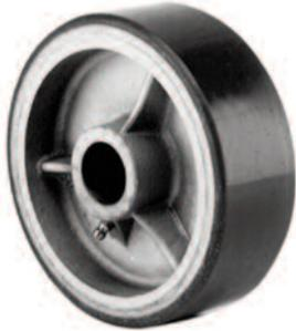
Polyurethane tread permanently attached to a metal core delivers a cushioned ride, excellent mobility and extended life under extremely heavy loads. Duro-Tred tires protect floors and loads better, will wear four to ten times longer than other wheel materials. Standard with roller bearings. Temperature operating range is +2°F to +180°F. Durometer rating is 95A.
