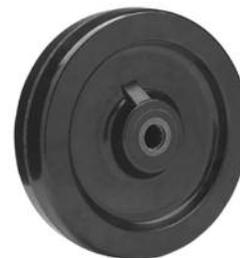
Phenolic compound reinforced with macerated fabric makes a high-strength, high-impact wheel resistant to oil, gasoline, even dilute acids. Compression-molded under extreme pressure, these wheels gain a dense, uniform consistency. Their smooth, chipless tread protects floors. Phenolic wheels are non-marking, non-conductive and spark-proof. Will not warp or swell in a temperature operating range of -40°F to +300°F. Durometer reading is 75D.
