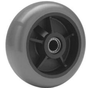
Thermoplastic rubber resists chemicals, caustics, oils, acids, and wear. Rugged polypropylene hub won't dent, mar, fade or stain. Tread and hub are double bonded and mechanically interlocked to eliminate tread separation. Gives dollies, carts and trucks a soft and cushioned non-marking ride. Temperature operating range is -40°F to +180°F. Durometer rating is 70A.
