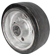
Press-on tires provide high capacities for extremely heavy loads. Both the rubber and polyurethane tread compounds provide long life and are highly resistant to chipping and abrasion. The treads are bonded to steel bands that are machine pressed onto fabricated or cast steel wheel centers. For added quality, these wheels also have large diameter tapered roller bearings.
