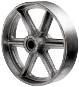
These cast iron wheels are toughened with steel to handle extremely high load ratings and provide exceptionally long life. They are recommended for rough wood and concrete floors, a good choice for moving heavy loads in manufacturing and warehousing. Long-life features include a heavy tread and roller bearings. Ideal in extreme operating temperature ranges of -40°F to +800°F with optional high temperature grease.
