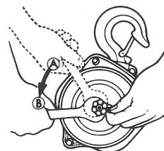
**Frequent Inspections** - Visual inspection by the operator or other authorized person. This inspection includes listening for unusual sounds while the hoist is operated that may indicate deficiencies.
