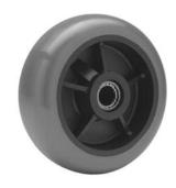
Thermoplastic rubber resists chemicals, caustics, oils, acids, and wear. Rugged polypropylene hub won't dent, mar, fade or stain. Tread and hub are double bonded and mechanically interlocked to eliminate tread separation. Gives dollies, carts and trucks a soft and cush-ioned non-marking ride. Temperature operating range is -40°F to +180°F. Durometer rating is 70A.
