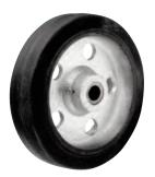
Cushioned rubber tread permanently vulcanized to a semi-steel core is recommended for quiet movement with heavy loads. Molded core provides added strength with a reinforced, double-thick hub. Vulcanized rubber-tread wheels are standardly supplied with roller bearings. Temperature operating range is -40°F to +158°F. Durometer rating is 75A.
