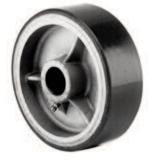
Polyurethane tread permanently attached to a metal core delivers a cushioned ride, excellent mobility and extended life under extremely heavy loads. Duro-Tred tires protect floors and loads better, will wear four to ten times longer than other wheel materials. Standard with roller bearings. Temperature operating range is +2°F to +180°F. Durometer rating is 95A.
