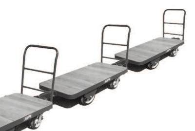
Caster steer trailers turn by swiveling on the front caster wheels. The casters have two full rows of large hardened balls for easy swiveling and proper lead to avoid whipping.
