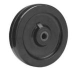
Phenolic compound reinforced with macerated fabric makes a high-strength, high-impact wheel resistant to oil, gasoline, even dilute acids. Compression-molded under extreme pressure, these wheels gain a dense, uniform consistency. Their smooth, chipless tread protects floors. Phenolic wheels are non-marking, non-conductive and spark-proof. Will not warp or swell in a temperature operating range of -40°F to +300°F. Durometer reading is 75D.
