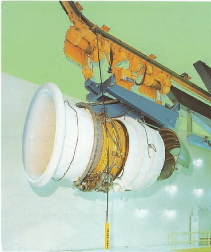
Louden monorail transports jet engine and spring beam into a test cell at an airline maintenance center, for automatic connection of wiring and plumbing.
