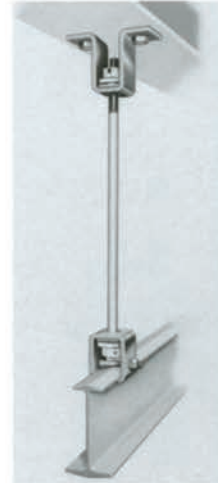
Used to connect Gimbal Rod assemblies to the bottom flange of superstructure beams. They are furnished complete with built-in hardened bearing washer and mounting bolts.
