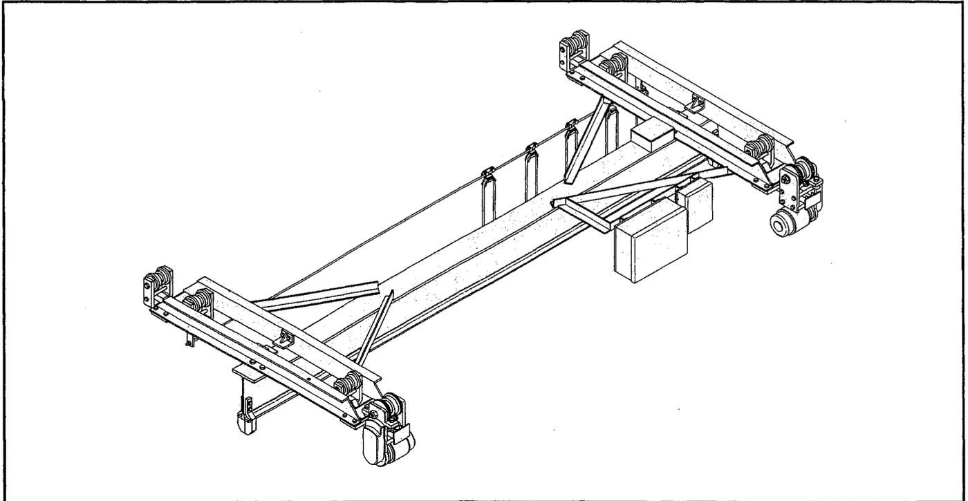
The Louden Series 585 steel wheel dual drive crane is offered in capacities of 1 through 5 tons, with spans to 50 feet. Standard bridge speeds are 75 and 125 F.P.M., single speed. Optional travel speeds (single speed) are 50, 100, 150 F.P.M. Also available in two speed and variable speed.
