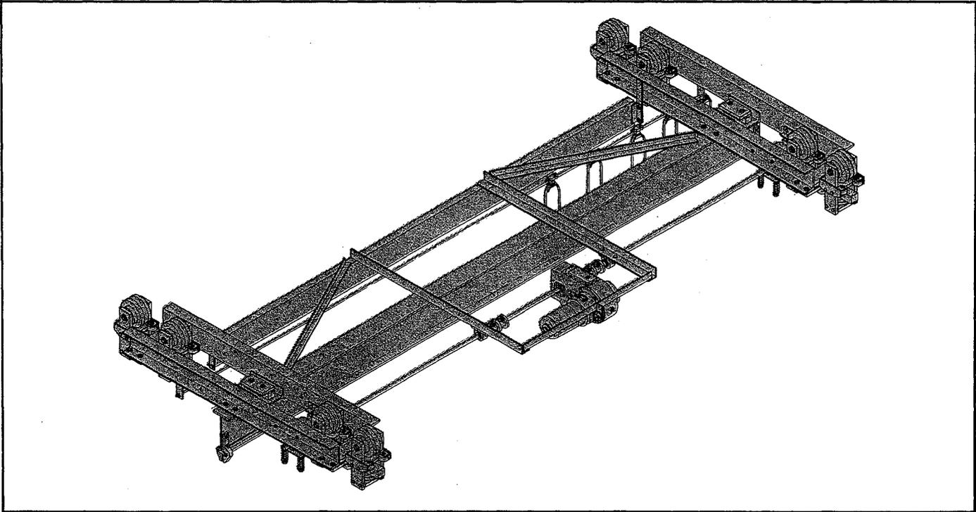
The Louden Series 503T center drive crane is offered in capacities of 5 through 10 tons, with spans to 60 feet. Standard bridge speeds are 75 and 135 F.P.M., single speed. Optional travel speeds (single speed) are 50, 110, 165, 190, and 255 F.P.M. Other optional speeds are 2-speed and variable speed. High speeds listed above.
