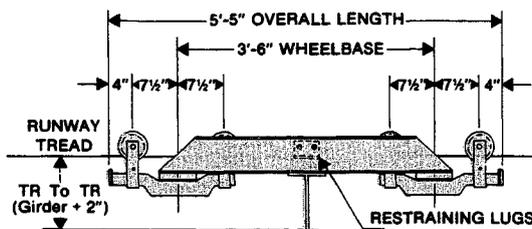
**8 Wheel, 6,000 lb. Cap. End Truck, with 3'-6" Wheelbase.**
