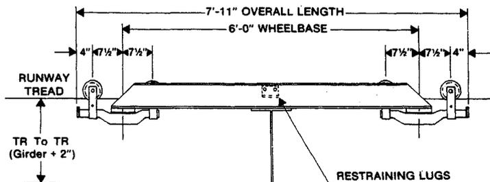
8 Wheel, 10,000 lb. Cap. End Truck, with 6'-0" Wheelbase.
