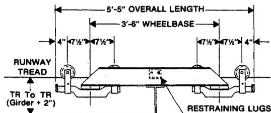
8 Wheel, 10,000 lb. Cap. End Truck, with 3'-6" Wheelbase.
