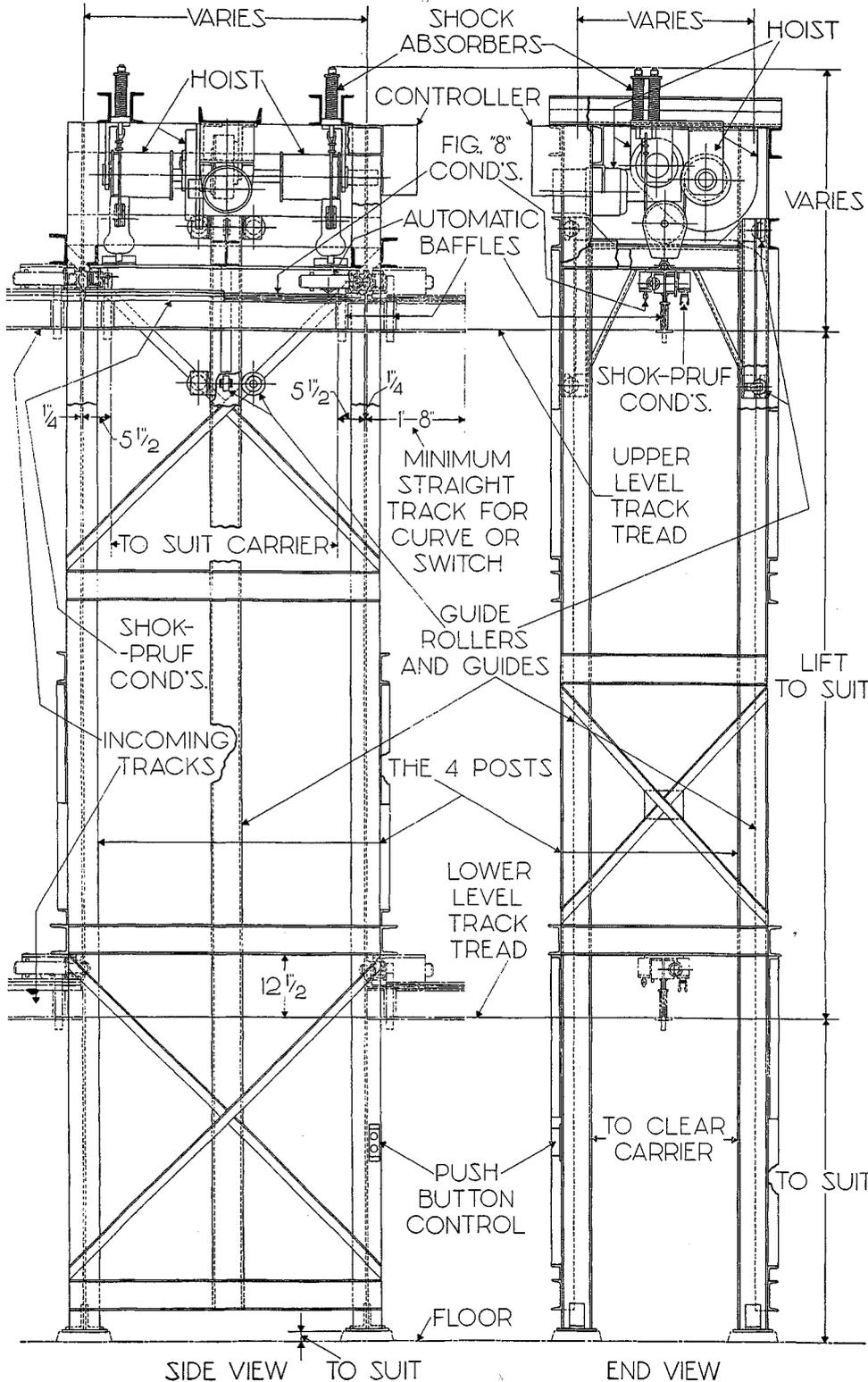
The four post, floor supported Track Hoist is used properly where there is no adequate overhead supporting structure, where the entire vertical travel must be guided, and where it is necessary for the live track section to align with tracks at two or more levels and at considerable difference in elevation. The four structural columns together with the hoist supports, aligning track supports and bracing, can be designed to be a completely self contained, self supporting structure.
