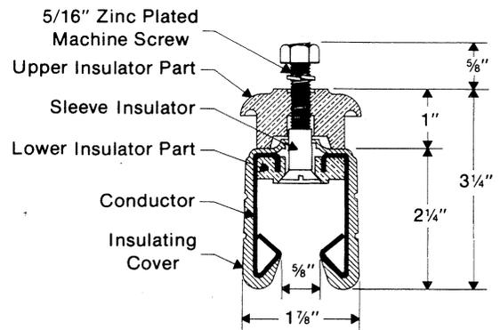
*Louden®* Dual Conductor Bottom Entry Electrification is stocked and shipped in standard 10' lengths; assembled complete with the specified insulating cover and five spacer insulators. When odd lengths are required as at the end of a run, the section is easily cut to length during installation.
