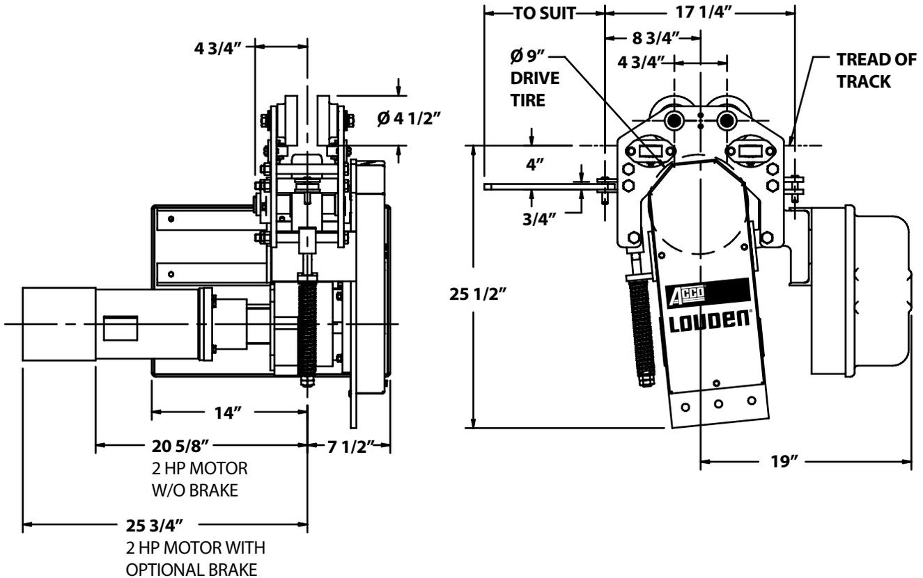
**Note:** The M9C is also available with the motor turned parallel to the direction of travel for applications where side clearance is limited. Contact the factory to discuss this application.
