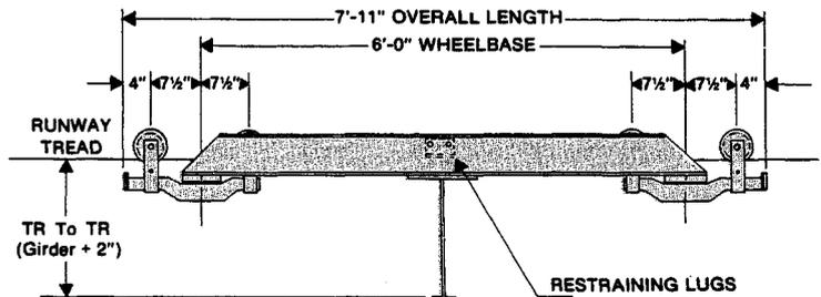
**8 Wheel, 6,000 lb. Cap. End Truck, with 6'-0" Wheelbase.**
