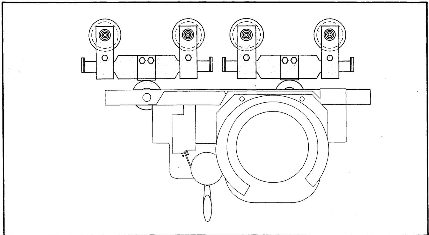
**8-Wheel, Cross Mounted, with Nose Piece Mounting
