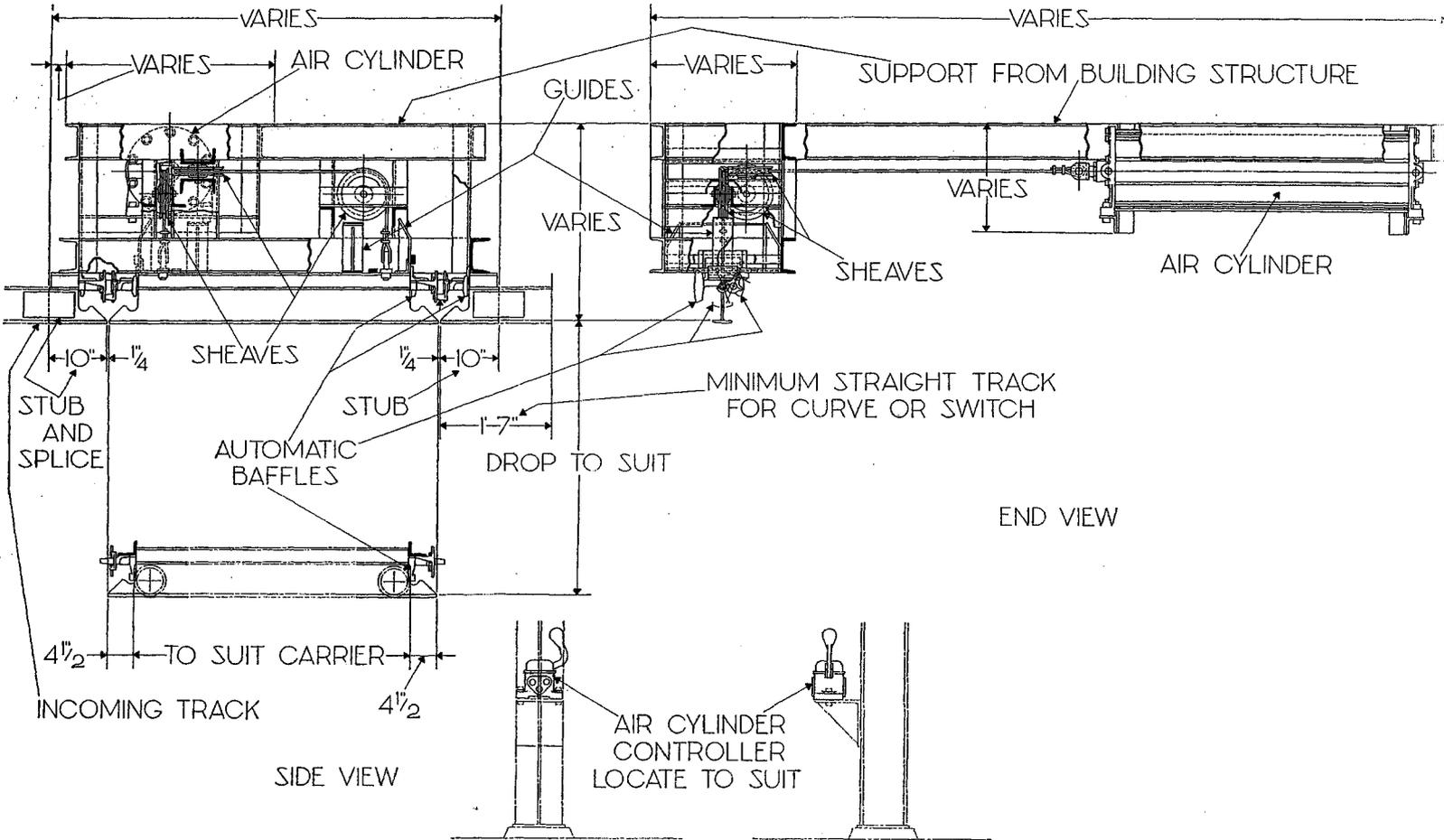
ited. Usually furnished with pneumatic or hydraulic cylinder hoists, the ceiling supported drop section can be equipped with an electric hoist which must be set to one side far enough to provide proper lead off drums and the directional sheaves in the Drop Section frame.
