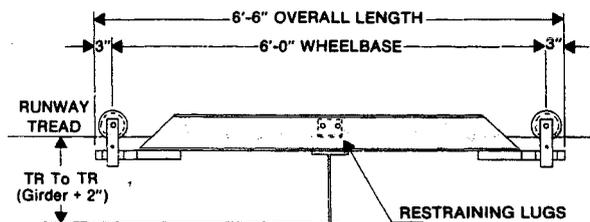
4 Wheel, 5,000 lb. Cap. End Truck, with 6'-0" Wheelbase.
