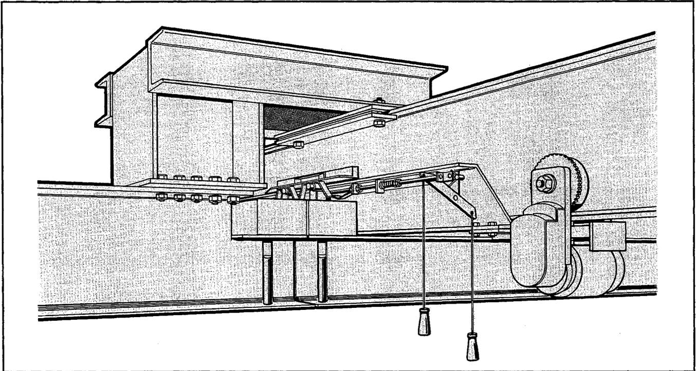
**Above illustration shows the No. 505.7824 Latch on the crane aligned and latched with the No. 504.7825 Latch Block on spur track.**
