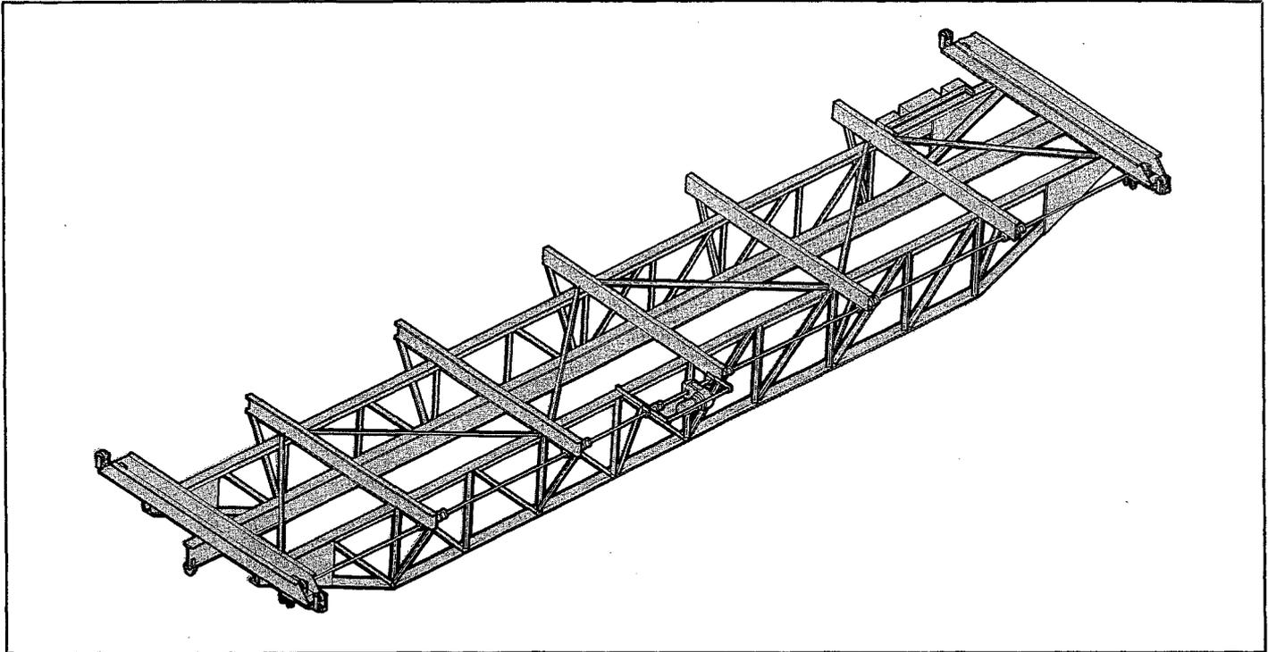
The *Louden* Series 510 and 510T center drive truss crane is offered in capacities of 3 through 15 tons, with spans to 100 feet. Standard bridge speeds are 75 F.P.M., single speed. Optional travel speeds (single speed) are 50, 110, 135, 165, 190, and 255 F.P.M. Other optional speeds are 2-speed and variable speed. High speeds listed above.
