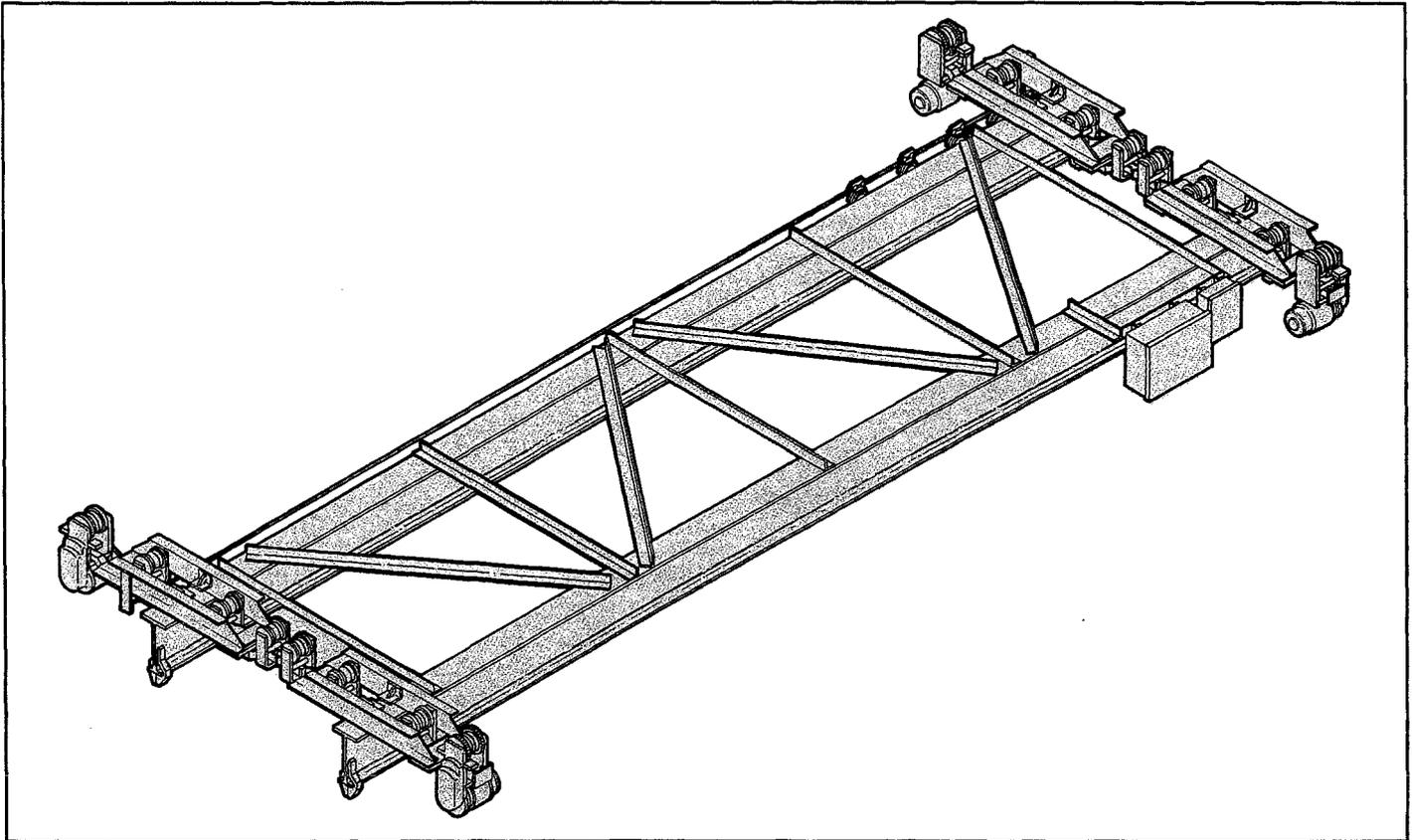
The Louden Series 586 double girder steel wheel drive crane is offered in capacities of 1 through 10 tons, with spans to 56 feet. Standard bridge speeds are 75 and 125 F.P.M., single speed. Optional travel speeds (single speed) are 50, 100, 150 F.P.M. Also available in 2-speed and variable speed.
