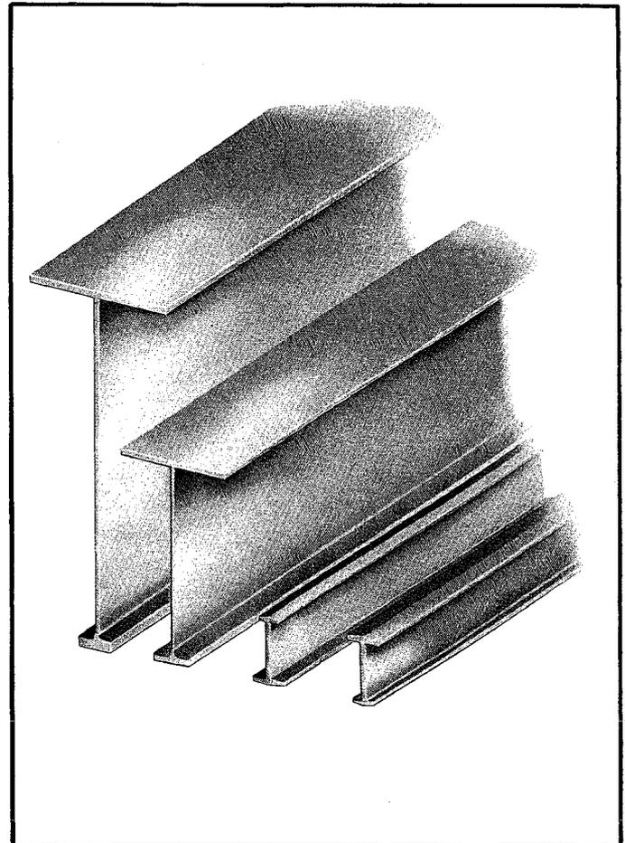
flange to give a load carrying member with a free span strength greater than *SuperTrack*™ Patented Track. The flat operating flange of *SuperTrack*™ Girder Track is 3.33" wide and 7/16" thick.
