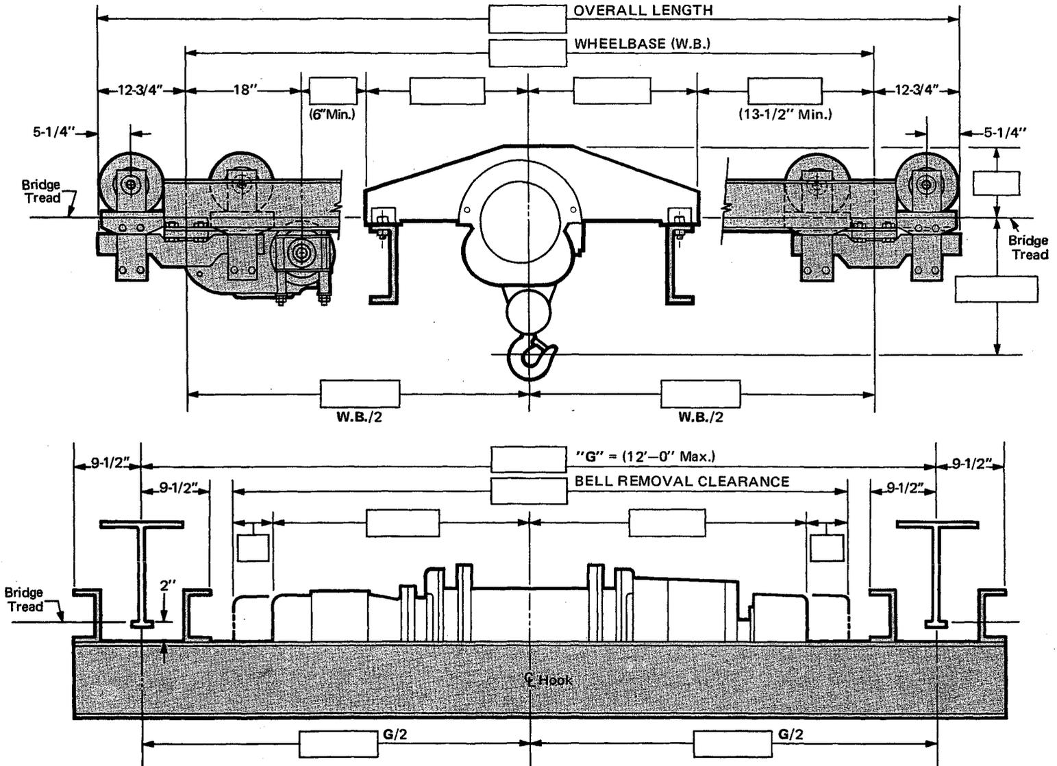
**NOTE:** All dimensions are approximate. Certified drawings will be supplied after completion of engineering.
