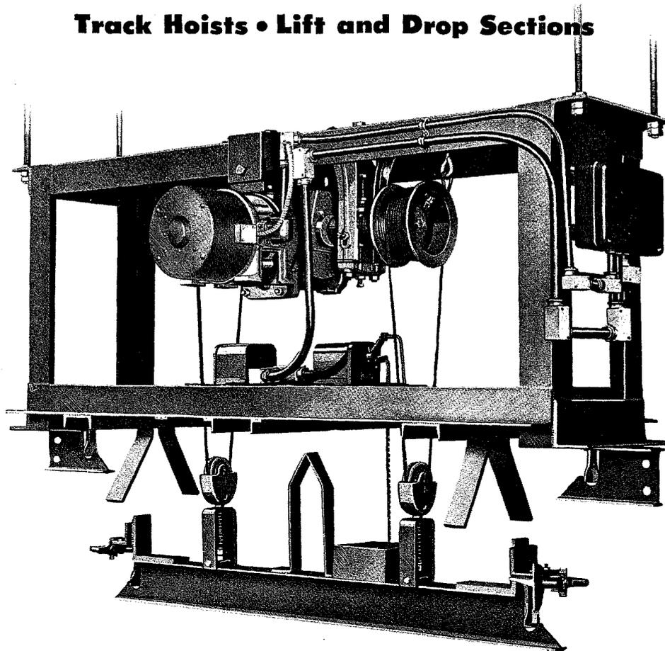
Many monorail systems requiring multiple carriers, and where hoisting occurs only at one or few fixed locations, can be installed with great economy by the use of Track Hoists, Lift or Drop Sections at the hoisting positions. Thus, the requirement for hoist equipment on each and every carrier is eliminated and the overall cost reduced accordingly.
