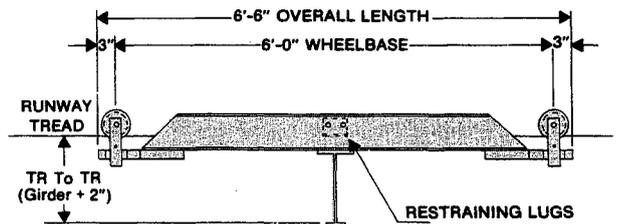
**4 Wheel, 3,000 lb. Cap. End Truck, with 6'-0" Wheelbase.**
