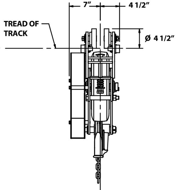
**M16 HAND CHAIN TRACTOR DRIVE WITH AUXILIARY REDUCER (NOT SHOWN)**
