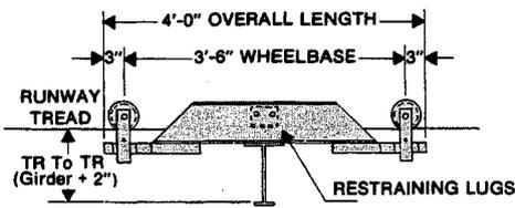
**4 Wheel, 3,000 lb. Cap. End Truck, with 3'-6" Wheelbase.**
