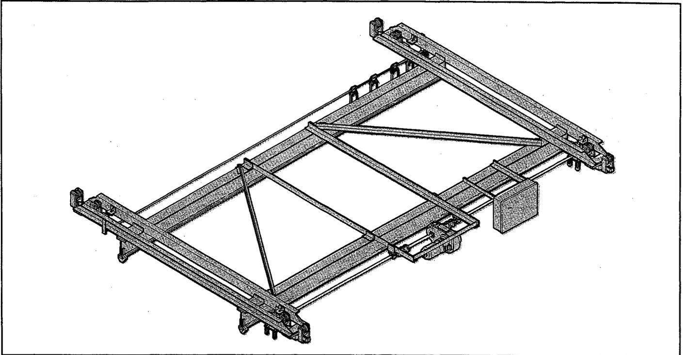
The Louden Series 517 center drive crane is offered in capacities of 1 through 10 tons, with spans to 60 feet. Standard bridge speeds are 75 and 135 F.P.M., single speed. Optional travel speeds (single speed) are 50, 110, 135, 165, 190, and 255 F.P.M. Other optional speeds are 2-speed and variable speed. High speeds listed above.
