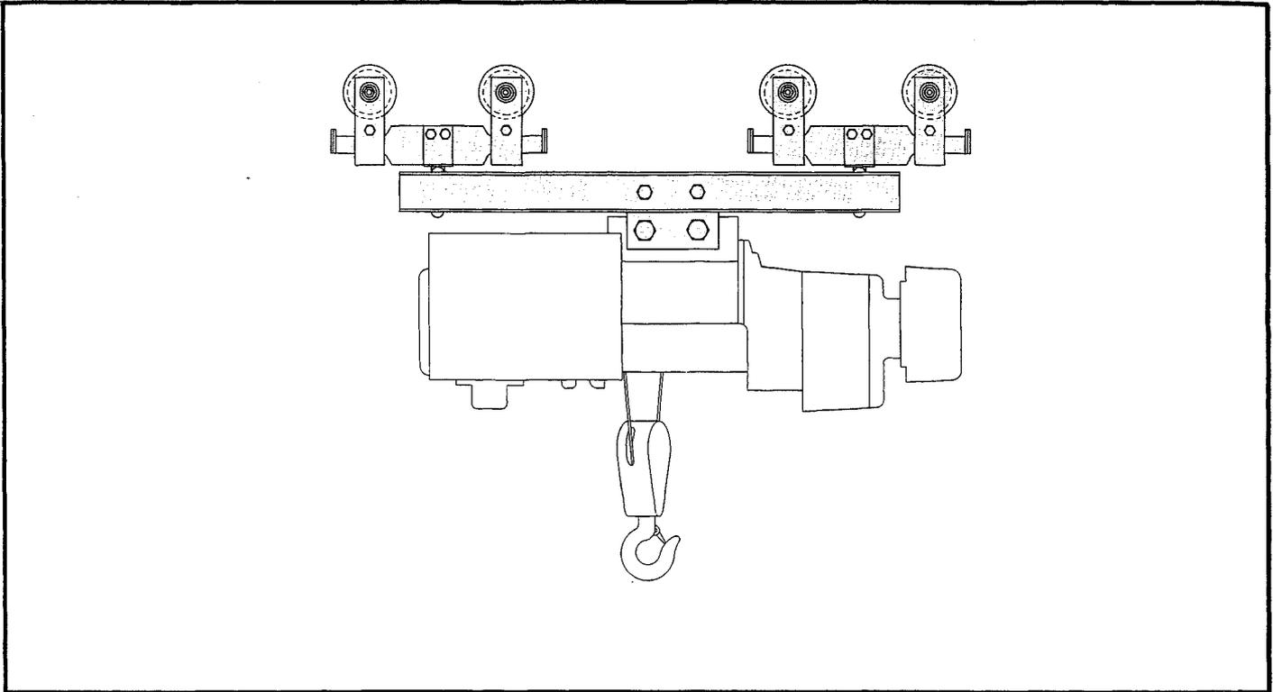
**8-Wheel, Parallel Mounted, with Bumper Protection
