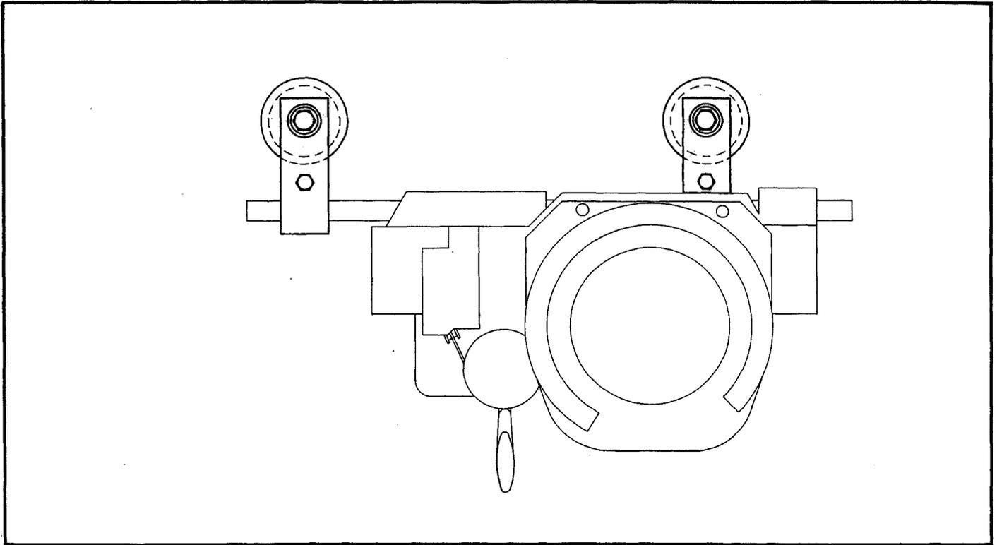
**4-Wheel, Cross Mounted with Nose Piece Mounting
