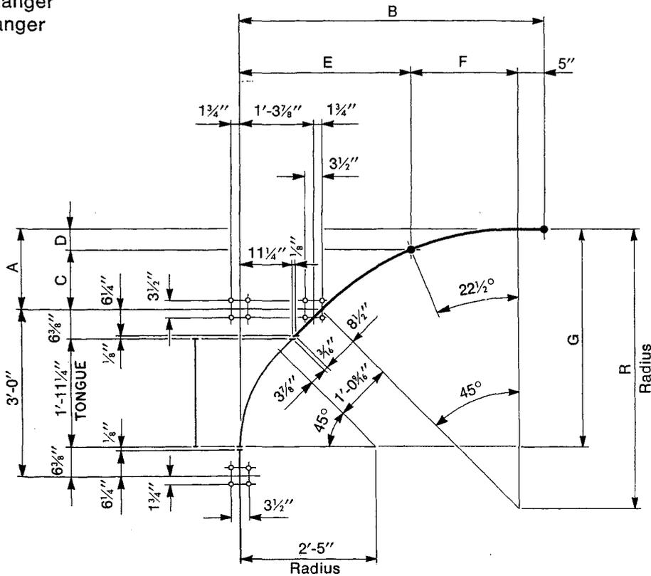
**Curve and Hanger Locations for Heavy Duty, Electrified SuperTrack Sliding Switches**
