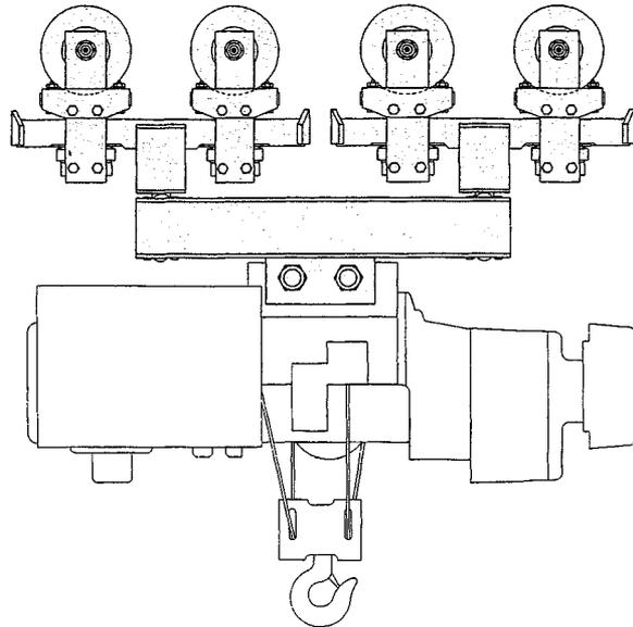
**8-Wheel, Parallel Mounted, with Bumper Protection
