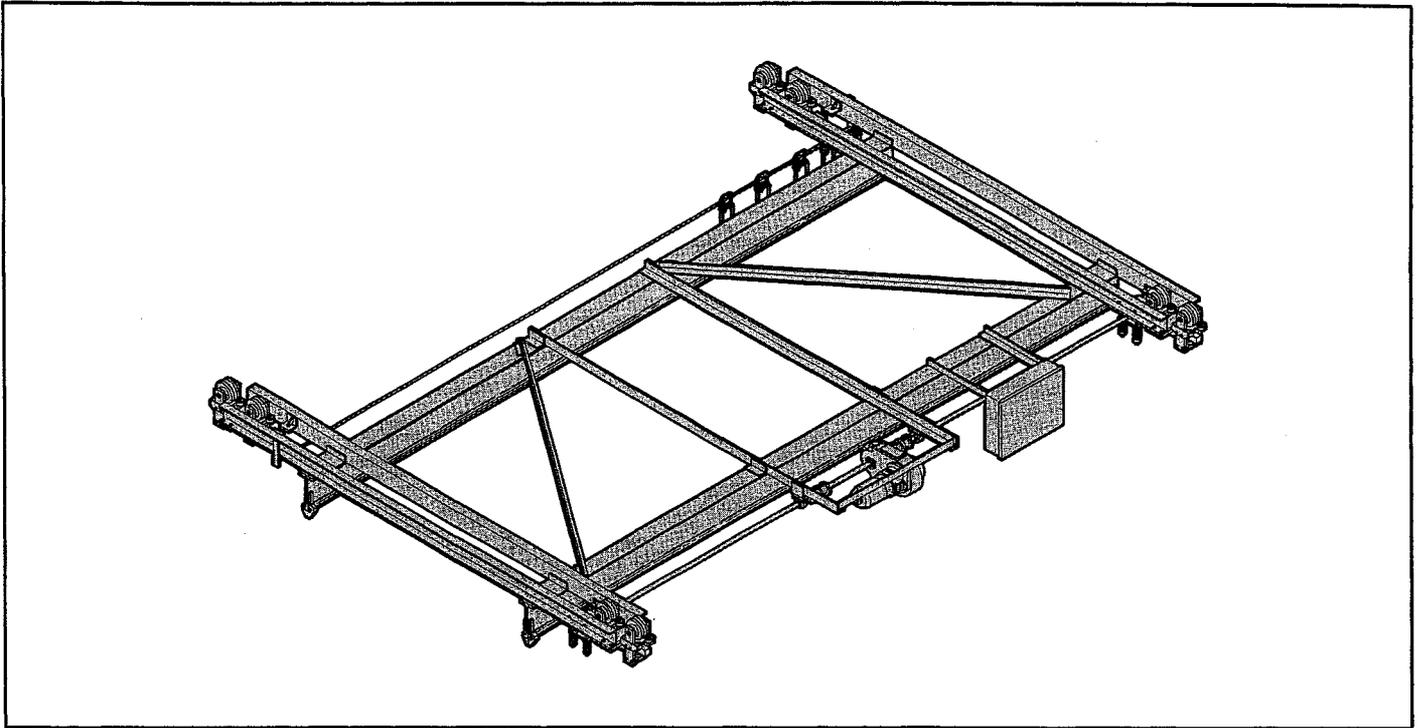
The *Louden* Series 517T center drive crane is offered in capacities of 5 through 10 tons, with spans to 60 feet. Standard bridge speeds are 75 and 135 F.P.M., single speed. Optional travel speeds (single speed) are 50, 110, 165, 190, and 255 F.P.M. Optional speeds are 2-speed, 3-speed and 5-speed will be accomplished through Variable Frequency Drives. High speeds listed above.
